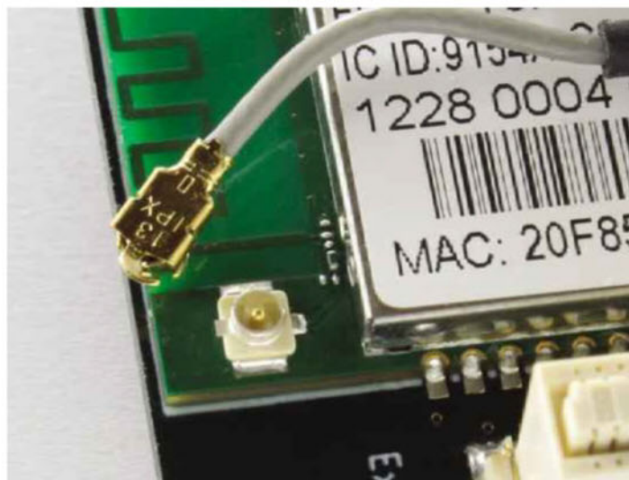
▲ The widely used Hirose U.FL coaxial connector
